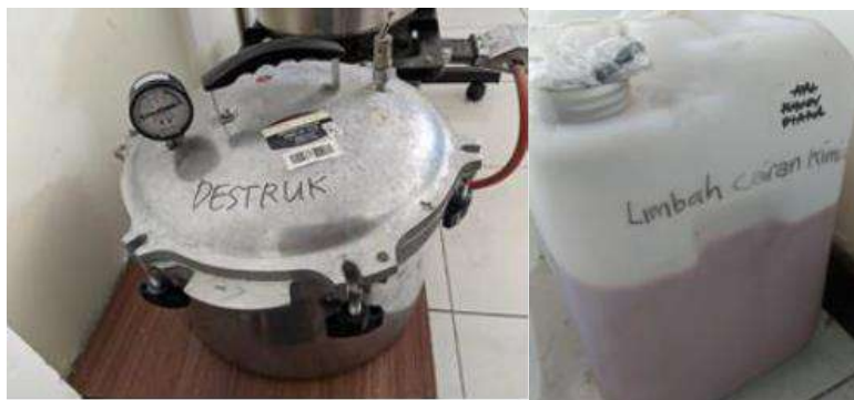
Figure 48. Autoclave and Liquid Solvent for Hazardous Waste
