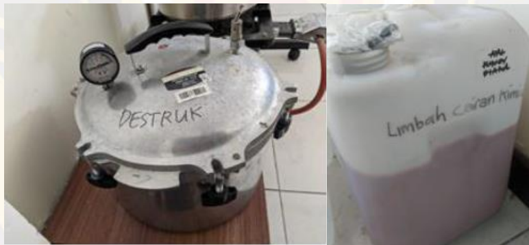
Figure 54. Autoclave and Liquid Solvents for Hazardous Waste
